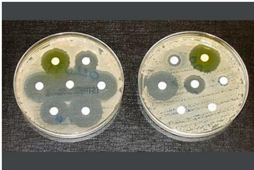
Antibacterial strength is determined by measuring the dead zone around the test substances in a Petri dish.
